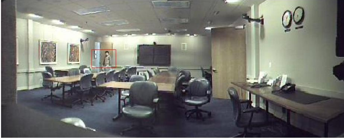
Fig. 6: Using image change to select a close-up view. The red region was automatically selected when the subject entered the room. Change of the clocks, however, was not detected.
