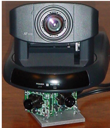
Fig. 1: The FlySPEC Camera: A pan-tilt-zoom camera (top) is combined with a fixed panoramic camera system (below.)
