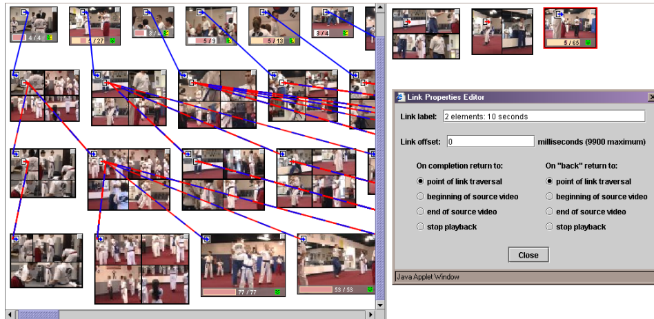
Figure 2: Editing a hypervideo summary. The left workspace is the automatically generated four-level summary. The right shows the components of one of the composites, allowing the components and their links to be modified.
