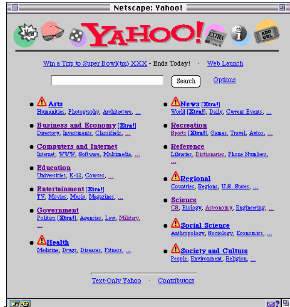
Figure 9: A document annotated with road sign icons to show hypertext anchors absent from the cache.
