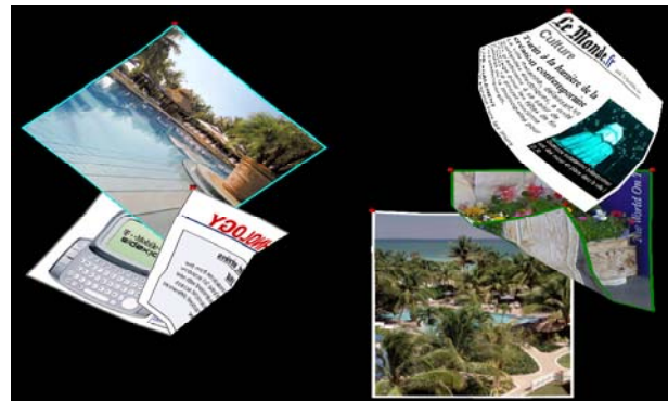
Figure 1. The Digital Bulletin Board runs on a touch-screen, showing folded fliers. Each flier is animated with a real-time cloth simulation. The textures are periodically refreshed over the network and remain interactive.
