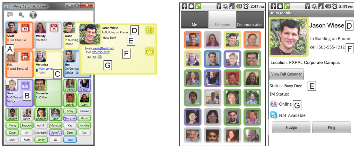
Figure 1. The desktop (left) and mobile (middle) dashboards. In addition to presence state, the desktop dashboard displays location from phone (A) or Bluetooth/Wi-Fi (C) as well as calendar information (B). The detail views for the mobile client (far right) and desktop (popup over dashboard) show presence data (D), status messages (E), contact information (F), and IM client status (G).
