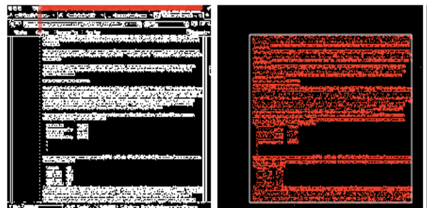
Figure 1. Left: binarized frame and red bars (top) showing the delta values computed with the previous frame. Right: image difference showing the bounding box (in white) used to restrict the region where the system computes the delta values for each column.
