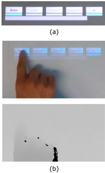
Figure 5: Projected UI of a custom toolbar with buttons. (a) View as seen by user (from a photo). (b) Video frames from RGB-D camera, color and depth. These images have been cropped to save space
