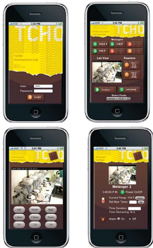
Figure 2. Screen shots from the iPhone app for controlling and monitoring machines in the chocolate development lab.
