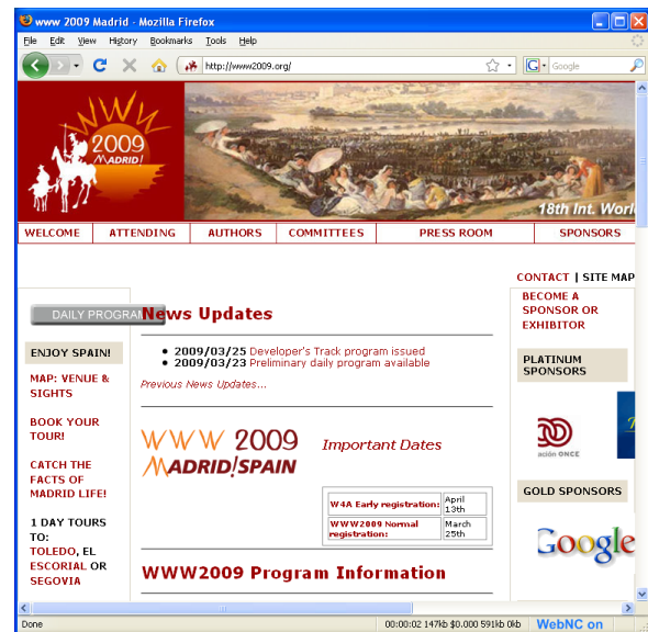
Figure 1. On the bottom right, the WebNC icon on reads “WebNC on” and is blue when the user shares a web browser window; otherwise, it reads “WebNC off” and turns black. Session time and bandwidth is shown left of the icon.
