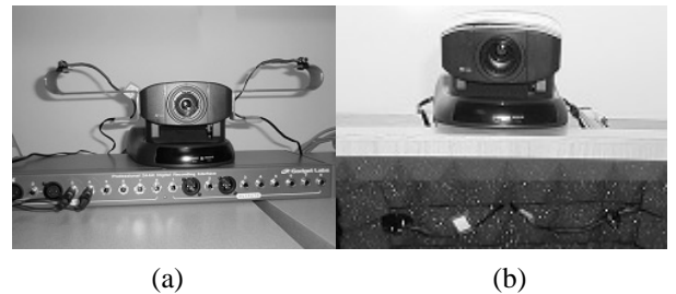
Figure 6. (a) Microphones are attached to extension structures of the active camera; (b) Microphones (lower portion of the figure) are separated from the active camera.
