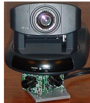
Figure 1. The FlySPEC Camera: A pan-tilt-zoom camera (top) is combined with a fixed panoramic multi-camera system (below)
