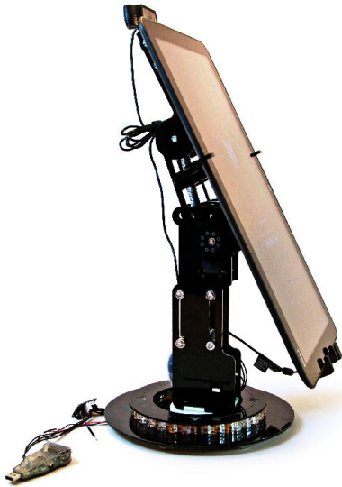
Figure 3. Jarvis: A desktop pan & tilt telepresence robot equipped with an 18" screen and HD video camera.
