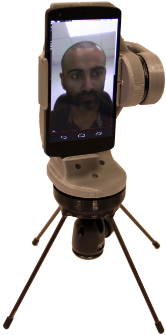
Figure 1: The current Polly prototype consists of a smart phone mounted on a three-axis brushless gimbal that can be carried, placed on perches or flat surfaces, or worn by the guide at shoulder level.
