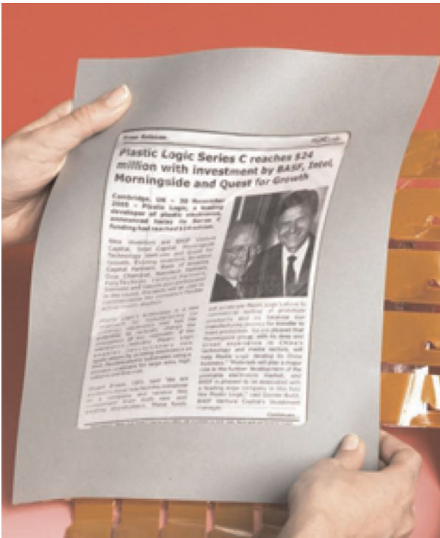
Fig. 3. Plastic Logic from E Ink Corporation: a flexible, high resolution, printed active-matrix backplane driving an electronic paper frontplane. Photo courtesy of E Ink Corp. press release. [A color version of this figure can be viewed online at journals.cambridge.org/aie ]
