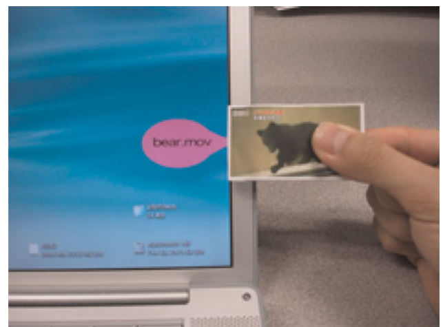
Fig. 9. A squeeze-it interaction function: squeezing the Post-Bit “squirts” a purple icon out onto the desktop; clicking the icon then brings up the movie clip. [A color version of this figure can be viewed online at journals.cambridge.org/aie ]
