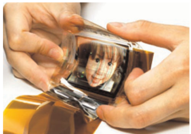
Fig. 2. Sony's video-rate flexible color e-paper in a 2007 demonstration. Photo courtesy of Sony Corp. press release. [A color version of this figure can be viewed online at journals.cambridge.org/aie ]
