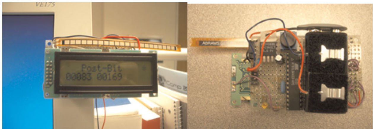
Fig. 12. (Right) A microcontroller prototype (Atmel, with LCD screen); (left) mounted to a display frame. [A color version of this figure can be viewed online at journals.cambridge.org/aie ]
