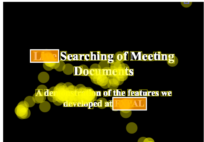
Figure 1. Detecting user actions on live meeting documents: yellow circles indicate detected mouse motion; white bordered rectangles show detected text selections
