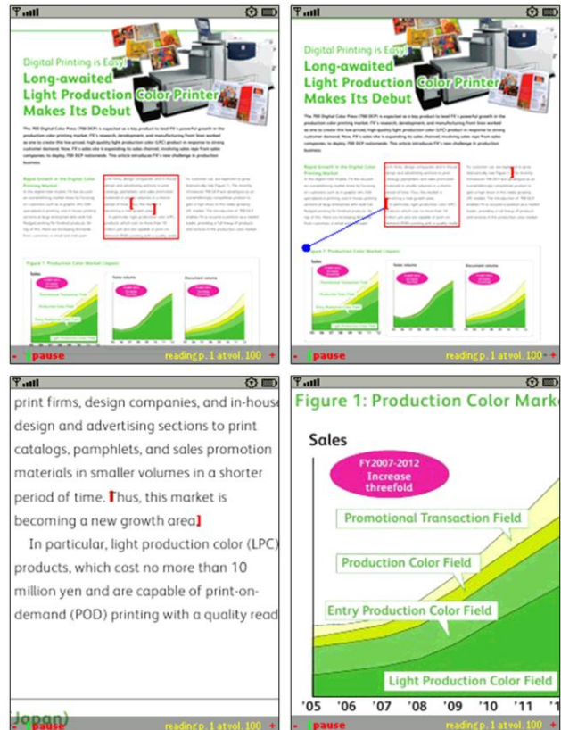
Figure 1: SeeReader automatically indicates areas of visual interest while reading document text aloud. The visual display shows the current reading position (left) before it encounters a link (right). When viewing the whole page, SeeReader indicates the link (top). When viewing the text, SeeReader automatically pans to the linked region (bottom). In both views, as the link is encountered, the application signals the user by vibrating the device.
