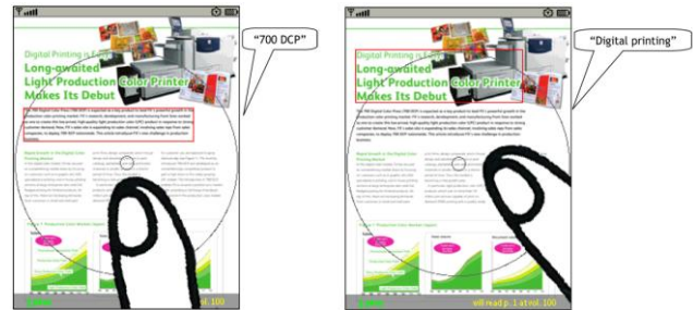
Figure 3: A user interacting with the touchwheel. As the user drags her finger around the center of the screen, the application vibrates the device to signal sentence boundaries and plays an audio clip of the keyphrase summarizing each region as it is entered.
